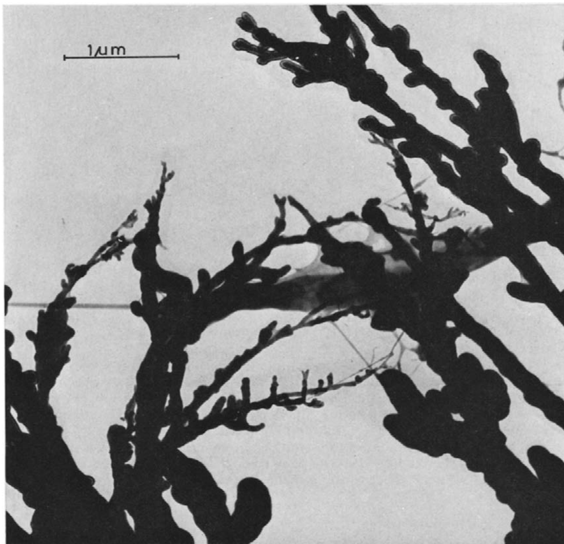
Fig. 1. Some of the micro-needles of a high-temperature activated emitter after dipping into a 0.001 M solution of a sample and evaporation of the solvent in the high vacuum of the ion source. (Electron micrograph by U. Nitschke, Bonn, G.F.R.).
